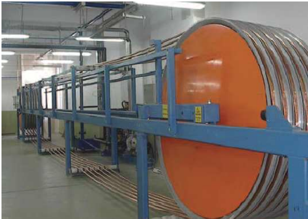
Accumulator in the CV-Line
