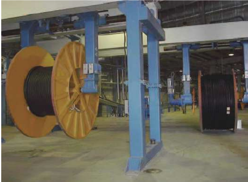
Pay-off Drums for triple extruded cables
