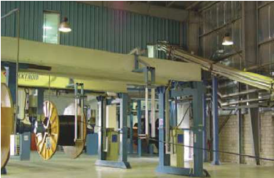
View of the CV-Lines tube that cross link the PE through dry or nitrogen curing
