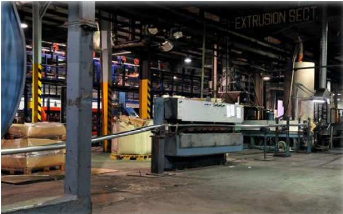
Outer Sheath/Jacketing Extrusion
